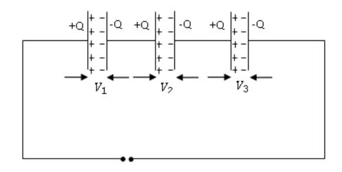
If the Capacitors are connected in Series the same charge 'Q' will be reaching to all the capacitors and the potential 'V' is divided into  $V_1$ ,  $V_2$  and  $V_3$  across  $C_1$ ,  $C_2$  and  $C_3$  respectively.
