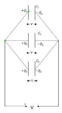
If the capacitors are connected in parallel, the potential difference across each capacitor will be same and equal to the source voltage, but the charge is distributed as  $Q_1$ ,  $Q_2$  and  $Q_3$  so that the charge from the source
