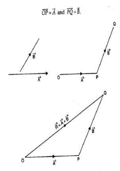
The sum of the resultant of  $\vec{A}$  and  $\vec{B}$  is represented by the vector  $\vec{OQ}$  (joining tail of  $\vec{OP}$  to the head of  $\vec{PQ}$ .
